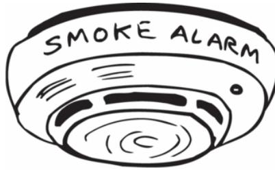
Smoke alarms should be installed in all sleeping areas, in hallways that lead to sleeping areas, and in each level of your home. Smoke alarms 10 years old or older should be replaced.
